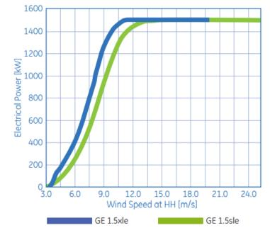
Figure 1: Reported Power Curves for 1.5 MW General Electric Turbines
