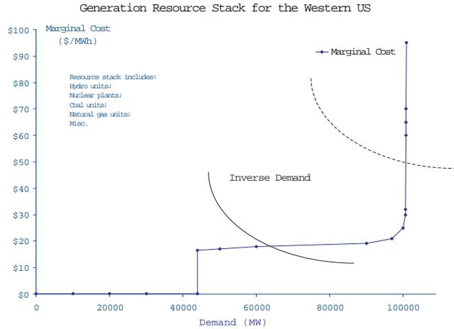
Figure 3: Generation Stack for Electricity in a Region
